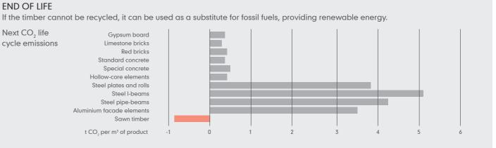
$CO_2$  can be saved using timber over the whole life cycle. Substituting 1m<sup>3</sup> of timber for other construction materials can result in savings of up to 1 tonne of  $CO_2$ . This combined with the carbon storage, means that 1m<sup>3</sup> of timber stores and substitutes 2 tonnes of  $CO_2$ .
